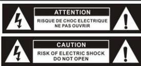
**CAUTION:** In order to reduce the risk of an electrical shock, do not remove any cover. There are no user-serviceable parts inside the device. Refer servicing to qualified service personnel only.
