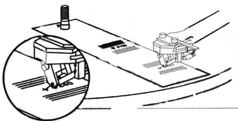
**VTA Adjustment:** To adjust the VTA, lay a record on the platter (15). Slacken the horizontal adjustment screws (two **Allen** screws located in the 11 and 1 o'clock position in the tonearm (10) base with the Allen Key provided.
