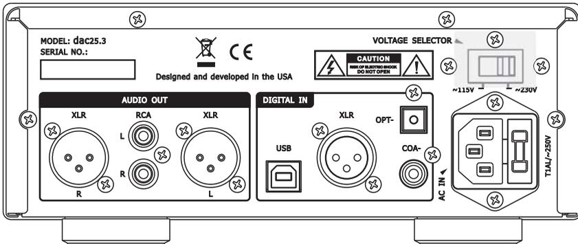
The dac25.3 has 4 digital inputs: coax (s/pdif), optical, USB, and XLR.
